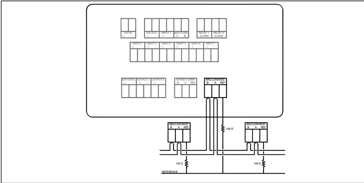
**Figure 33. Optional Modbus and BACnet MS/TP Communications Wiring to Model RPM10/RPM20**
