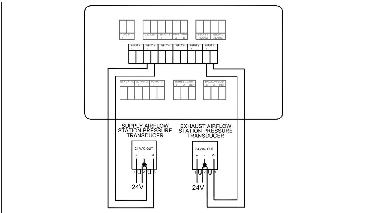
**Figure 23. Optional Supply/Exhaust Pressure-Based Flow Station Wiring to Model RPM10/RPM20**
