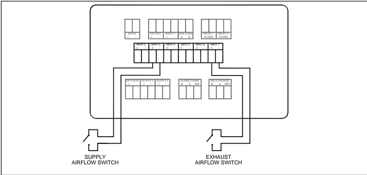
**Figure 22. Optional Supply / Exhaust Flow Switch Wiring to Model RPM10/RPM20**
