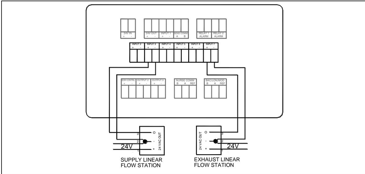
Figure 24. Optional Supply/Exhaust Linear Flow Station Wiring to Model RPM10/RPM20
