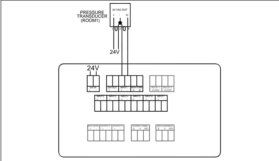
Figure 20. Pressure Transducer Sensor Wiring to Model RPM10/RPM20
