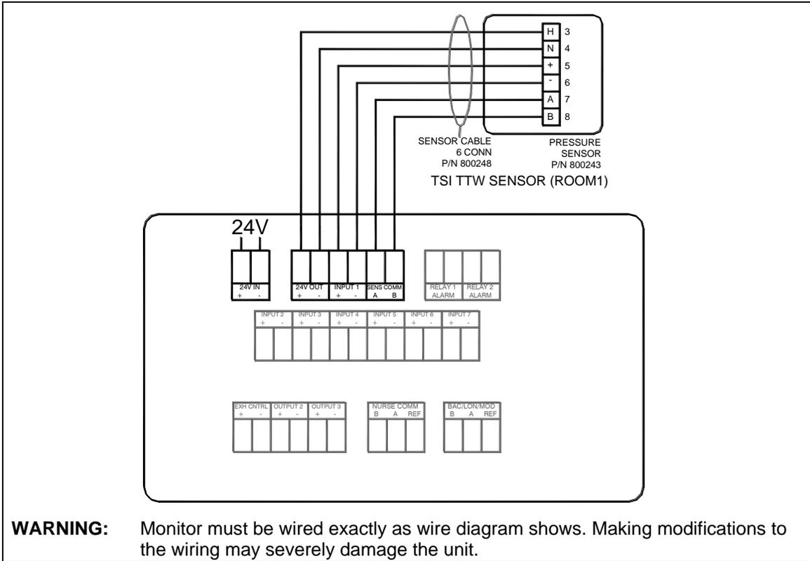
**WARNING:** Monitor must be wired exactly as wire diagram shows. Making modifications to the wiring may severely damage the unit.
