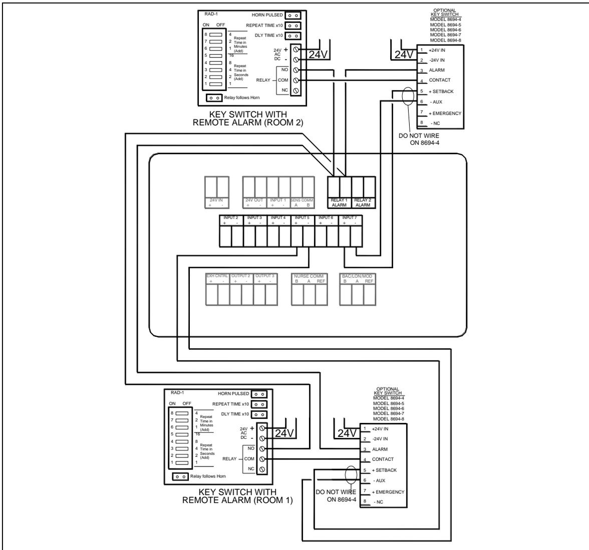
Figure 30. Optional Keyswitch with Remote Alarm Wiring to Model RPM10/RPM20
