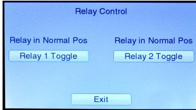
Figure 14. Relay Outputs screen in Diagnostics menu
