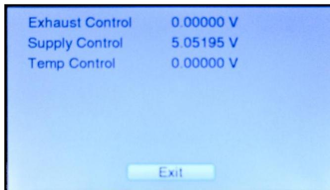
Figure 16. View Outputs screen in Diagnostics menu
