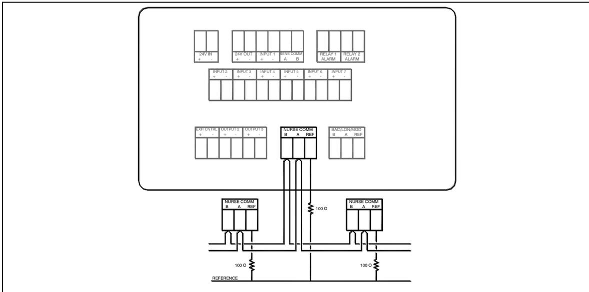
Figure 32. Optional Nurses Station Communications Wiring to Model RPM10/RPM20
