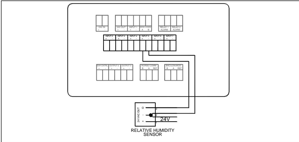
Figure 31. Optional Relative Humidity Sensor Wiring to Model RPM20
