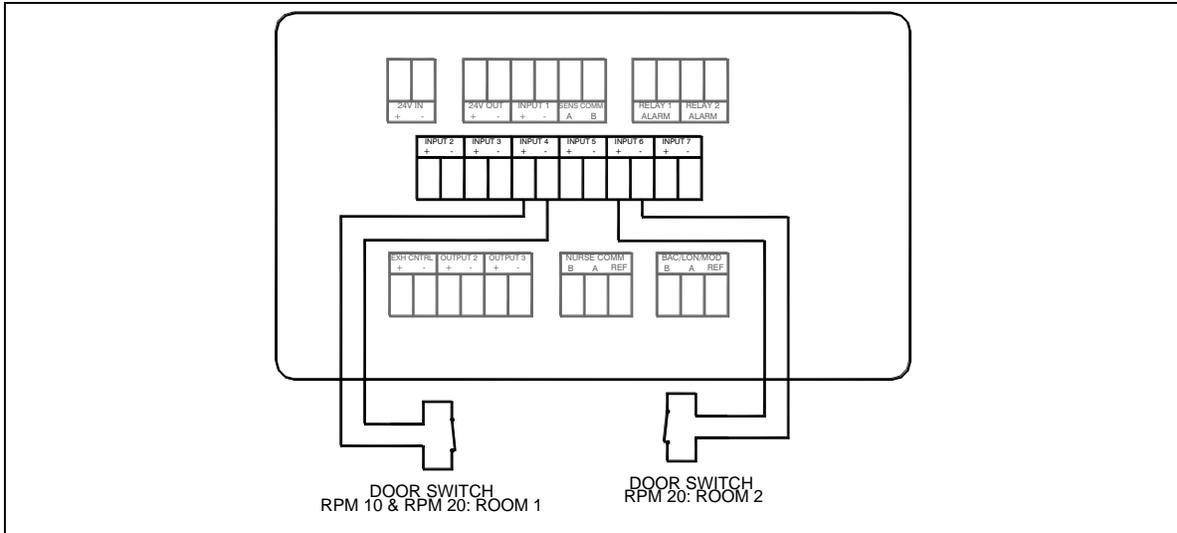
**Figure 26. Optional Door Switch Wiring to Model RPM10/RPM20**
