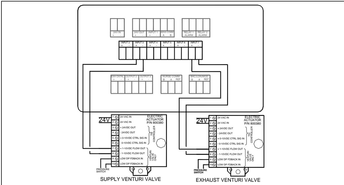
Figure 25. Optional Supply/Exhaust Venturi Valve Wiring to Model RPM10/RPM20
