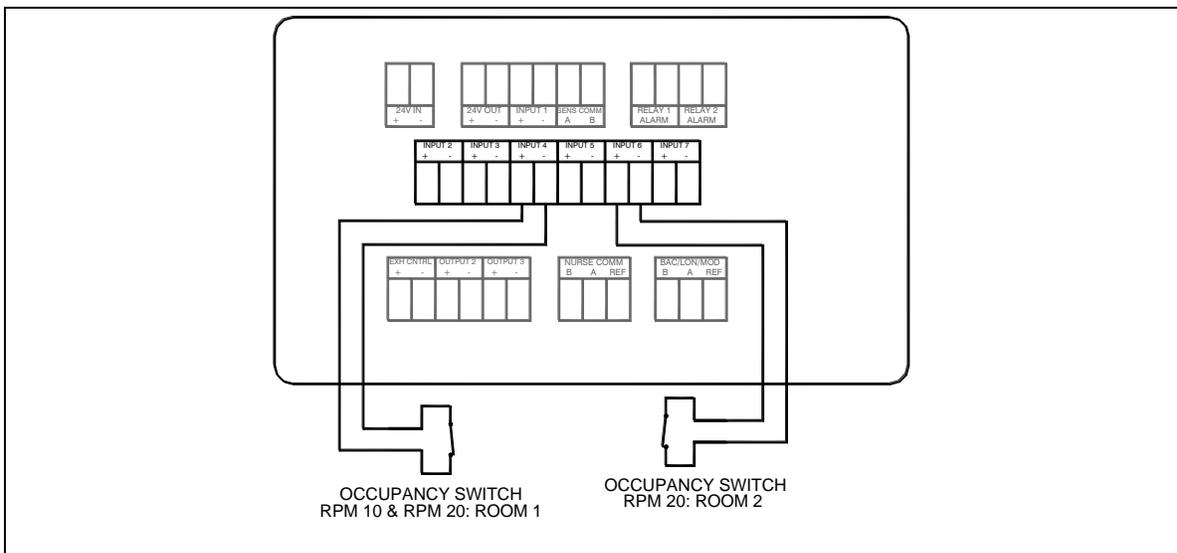
**Figure 27. Optional Occupancy Sensor Wiring to Model RPM10/RPM20**
