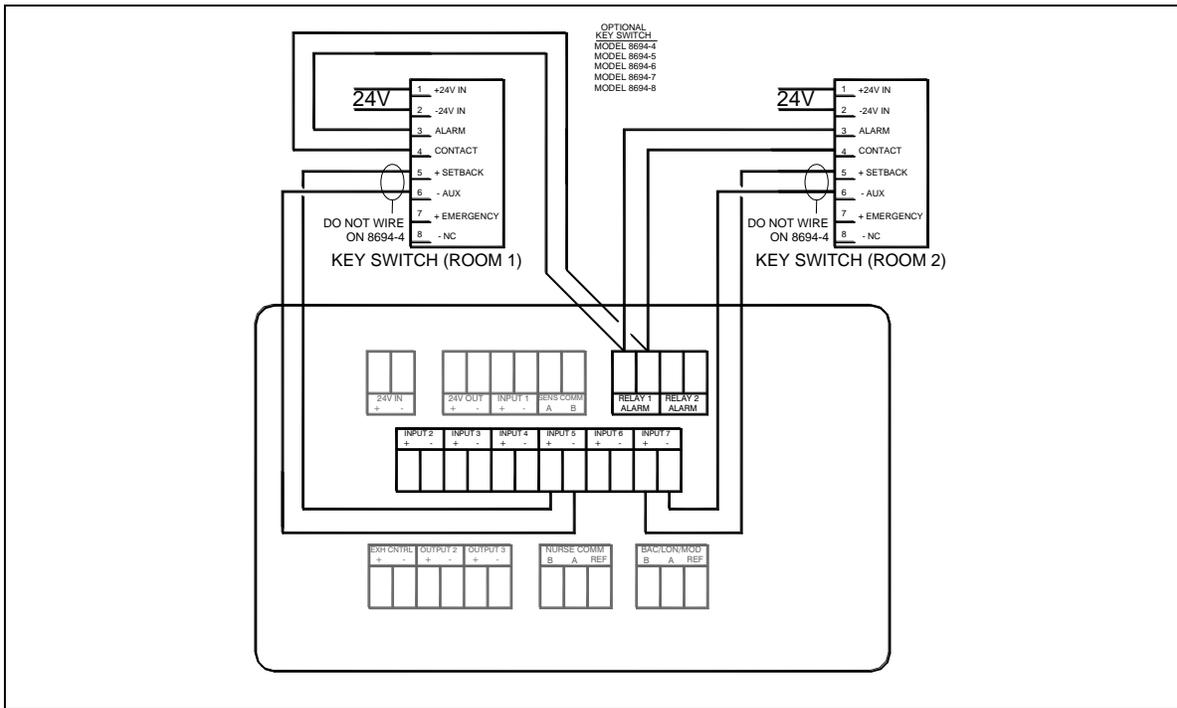
Figure 29. Optional Keyswitch Wiring to Model RPM10/RPM20
