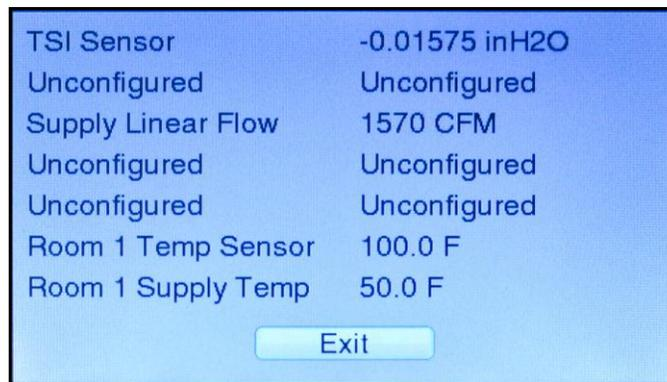
Figure 15. View Inputs screen in Diagnostics menu
